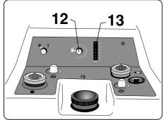
Cold water mode 0 - 50°C Hot water mode 50 - 95°C Steam mode 95 - 150°C
