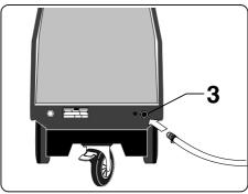
Min length of hose: 6 m. 3/4". Clean water inlet filter (3) at monthly intervals.
