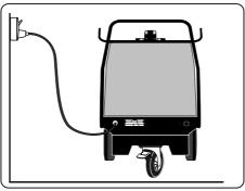
Only connect to an approved socket with earth connection.
